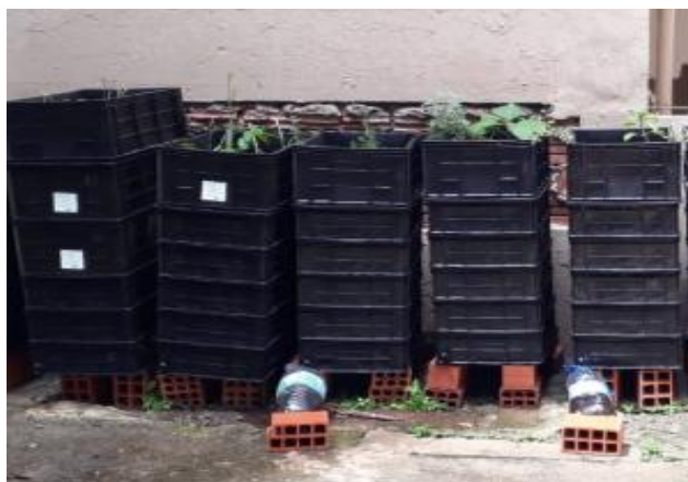
Figure 2. Gallons of 5l for leachate withdrawal.
